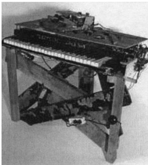
Plate 6.14 Electronic Sackbut prototype, invented by Hugh Le Caine in 1948. This was the first voltage-controlled analog synthesizer. (© Hugh Le Caine Archive, National Research Council Canada)
