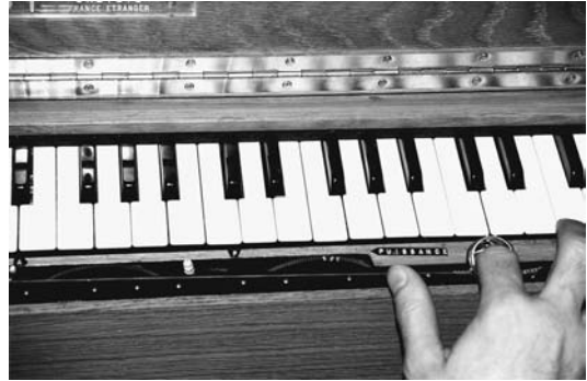
Plate 1.13 Ondes Martenot: right hand showing view of finger-ring controller. (Photo by Thom Holmes)
