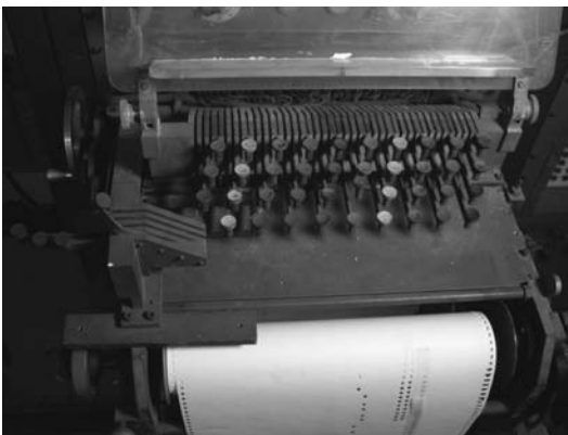
Plate 6.3 Punched paper recorder/reader of the RCA Mark II. (Photo by Thom Holmes)
