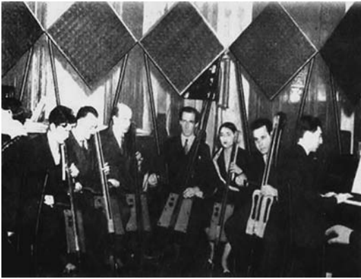
Plate 1.9 An ensemble of cello Theremins, 1932. The monophonic instrument was played by pressing a finger to the plastic fingerboard to produce a note. A handle was used to adjust volume. Behind the performers are pictured several diamond-shaped loudspeakers.
