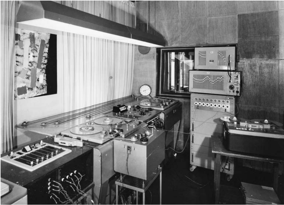
Plate 2.4 A section of the WDR Studio for Electronic Music, Cologne, in 1966, when Stockhausen was composing Hymnen . From left: corner of a four-track tape recorder; mixing console; mono tape recorder; Springer (in front of the mono tape recorder) with rotating head for suspending sounds; board with six roller guides for long tape loops; switching board with three sliding faders; sound meter; large stopwatch; second mono tape recorder; nine-octave filter; two Albis filters; portable Telefunken M5 tape recorder. (Stockhausen Verlag)
