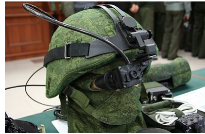
1PN139 thermographic monitor, and protective headgear from the 6B49 suit.
