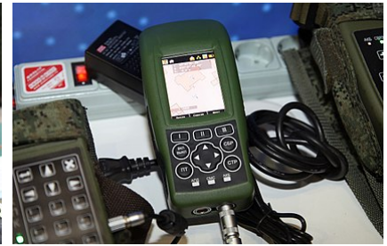
NPI-2 wearable GLONASS receiver for the soldier.
