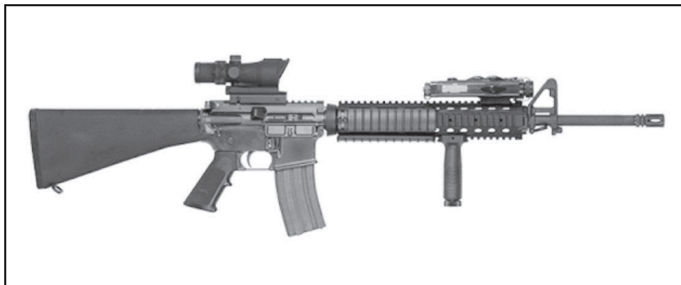
Figure 4-5. Vertical foregrip example
