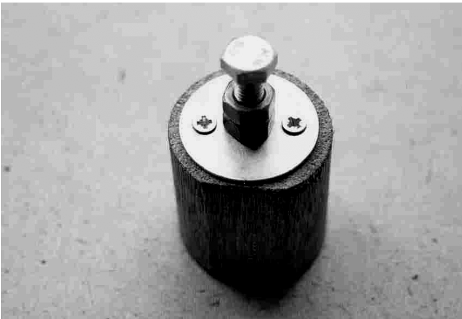
The finished seating die.
