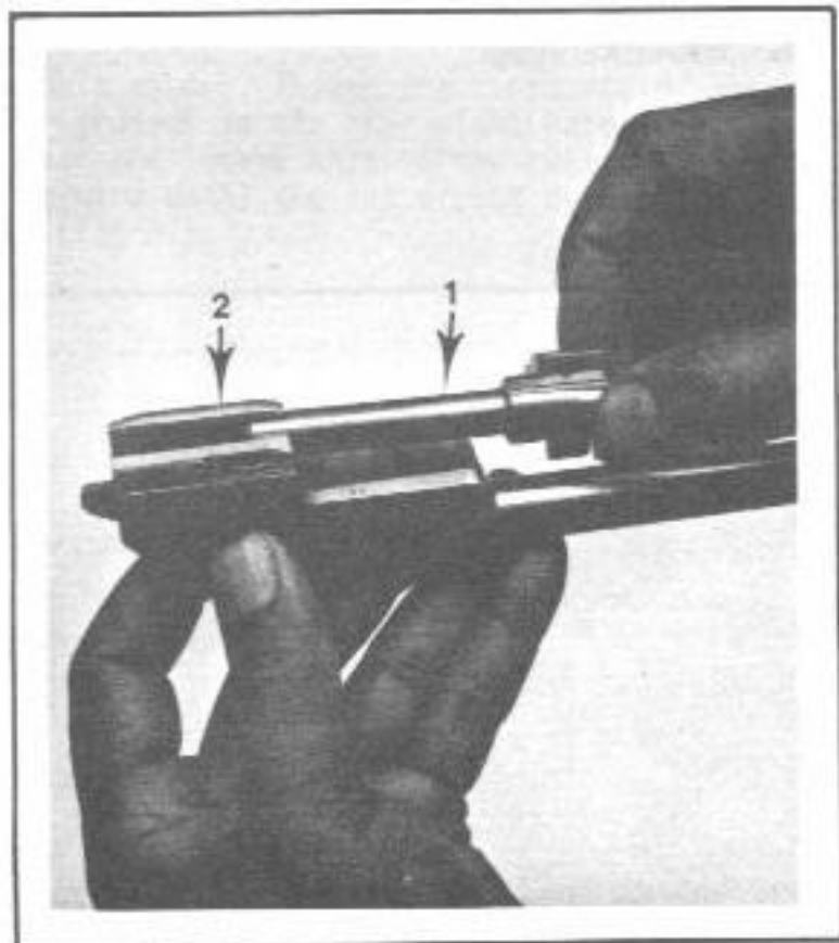
FIGURE 38. REPLACING THE BOLT
