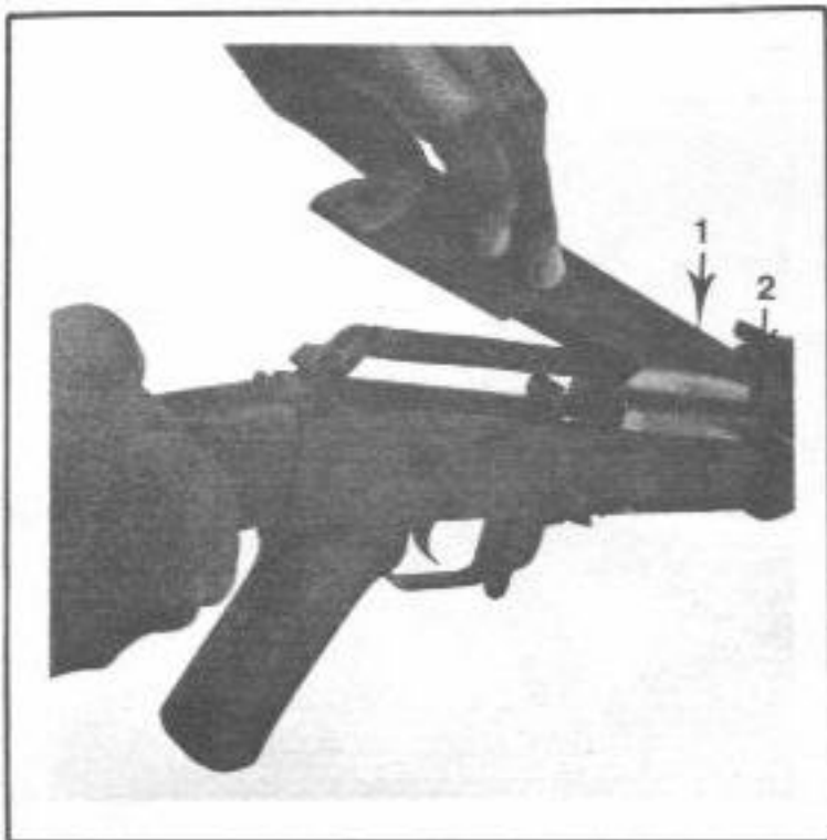
FIGURE 45. REPLACING BOLT COVER
